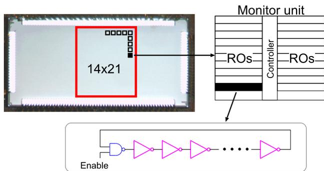
Fig. 9 Test chip structure. several types of ROs are implemented on-chip.
