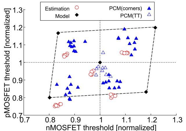
**Fig. 12** Comparison between threshold voltages in corner model and in estimations. PCM data for “TT” corner wafer as well as other corners are also plotted.**Table 3** Extracted standard deviation of MOSFET threshold voltages and gate length from RO frequency measurements.
