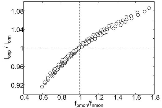
**Fig. 8** Correlation between MOSFET ON-current ratio,  $I_{onp}/I_{onn}$  and monitor frequency ratio ( $f_{pmon}/f_{nmon}$ ). High correlation coefficient of 0.98 is found. The p- and n-monitors can detect P/N-ratio with high accuracy.
