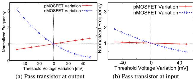
**Fig. 4** Sensitivity to MOSFET threshold voltage variation. Structure of (b) is sensitive to particular MOSFET variation thus suitable for parameter extraction.
