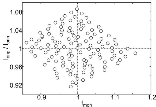
**Fig. 7** Correlation between ON-current ratio of MOSFETs,  $I_{onp}/I_{onn}$  and standard inverter based process monitor frequency.
