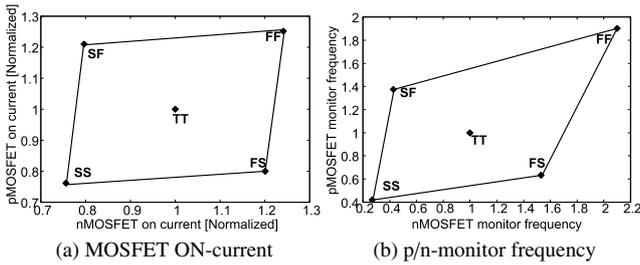
**Fig. 6** MOSFET ON-currents (a) and monitor frequencies (b) simulated at the process corners. Monitor frequencies are distributed in the process space.
