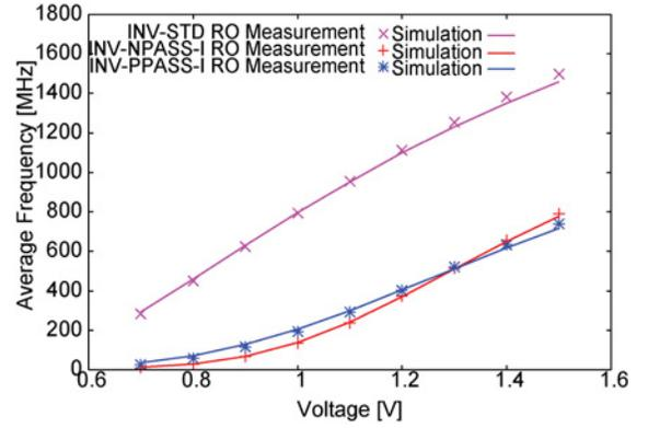
Fig. 19. Measured average frequency and simulated frequency of homogeneous ROs. Simulation is performed at the estimated center point in the process corner.
