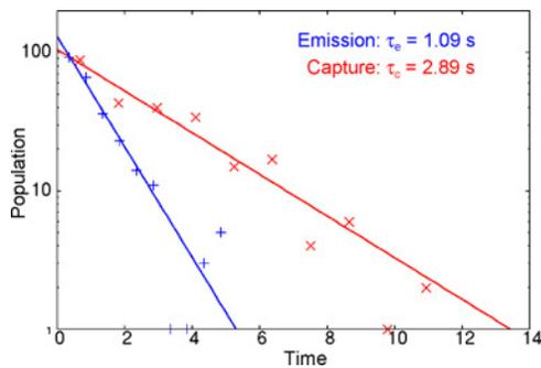
Fig. 23. Time constants of emission and capture time calculated from Fig. 21.
