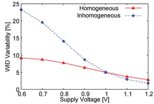
Fig. 12. Comparison between WID random variabilities of homogeneous “INV-NPASS-I” and inhomogeneous “INV-NPASS-I” RO at different supply voltages. The effect of inhomogeneity increases with decrease of supply voltage.
