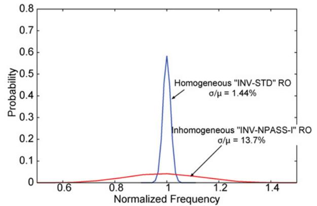
Fig. 11. RO frequency distribution at 0.8 V supply. Large variation is observed for inhomogeneous “INV-NPASS-I” RO.
