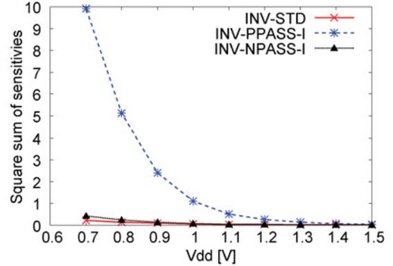
Fig. 16. Square sum of sensitivities to  $V_{thP}$  variation against supply voltage for different ROs.
