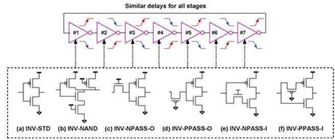
Fig. 1. Conventional seven-stage RO structure where the same type of inverter structures are used for all stages. As the RO oscillation period is the sum of each inverter stage delay, variation in a particular stage is not directly visible.
