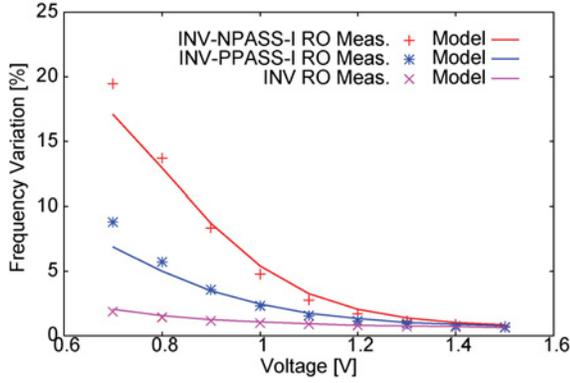
Fig. 20. Estimated frequency variations and measured frequency variations for three different ROs. Model Eq. (6) is used to estimate frequency variations using extracted variations of  $V_{thP}$ ,  $V_{thN}$  and  $L$ .
