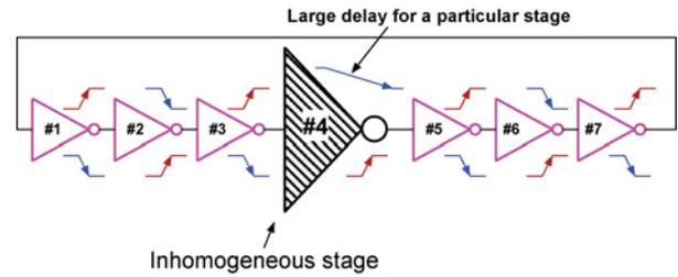
Fig. 2. Proposed inhomogeneous RO structure. A particular stage is designed to have a large enough delay compared to other stages so that the output frequency is a strong function of that particular stage's delay. Any variation in the inhomogeneous stage becomes directly visible to the output frequency.
