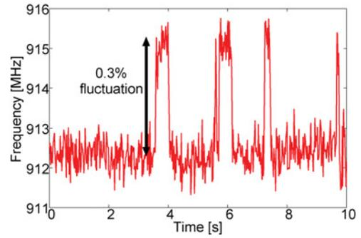
Fig. 15. RO frequency for an “INV-NPASS-I” inhomogeneous RO circuit over 10 s with binary fluctuation (RTN) at 1.2 V supply.
