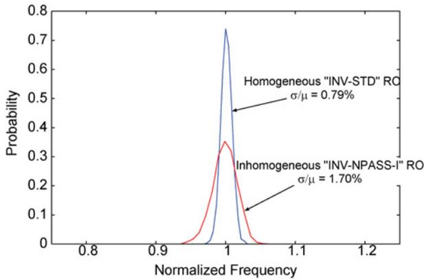
Fig. 10. RO frequency distribution at 1.2 V supply.
