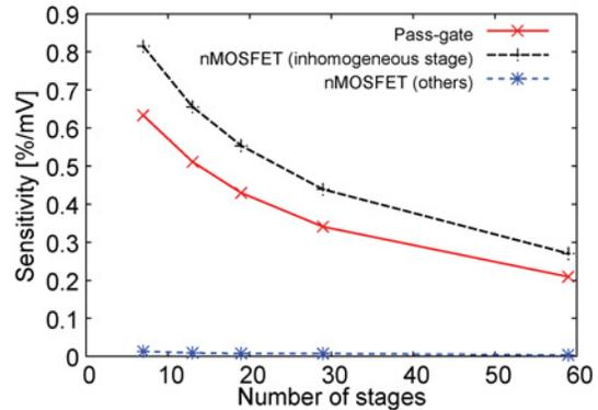
Fig. 8. Change of frequency sensitivity to individual transistor variation against the number of stages. Increase in the number of stages reduces the sensitivities of the transistors in the same proportion.
