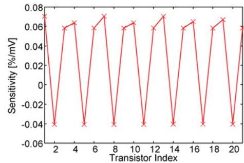
Fig. 3. Sensitivity of each transistor in a seven-stage homogeneous RO with conventional nMOSFET pass-gate loaded inverter. Similar sensitivities are observed for the MOSFETs in each inverter stage.
