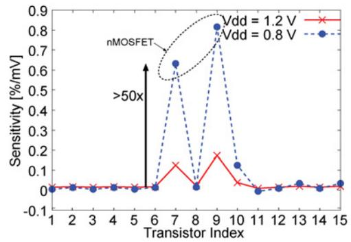
Fig. 7. Sensitivity of each transistor in a seven-stage inhomogeneous RO of Fig. 6.
