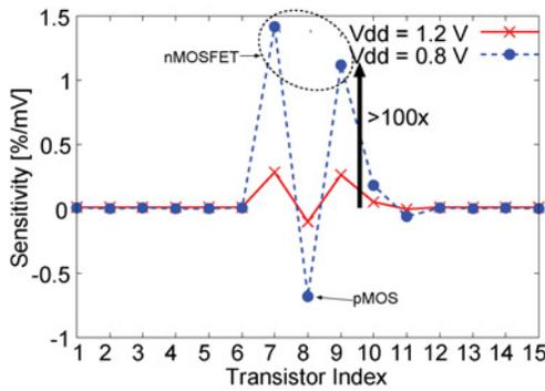
Fig. 5. Sensitivity of each transistor in a seven-stage inhomogeneous “INV-NPASS-O” RO of Fig. 4.
