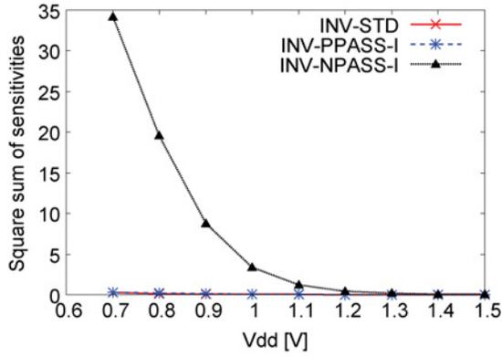
Fig. 17. Square sum of sensitivities to  $V_{thN}$  variation against supply voltage for different ROs.
