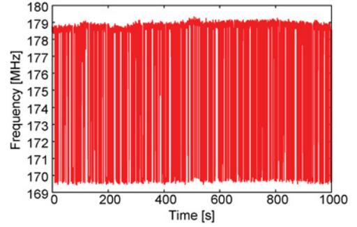
Fig. 21. Frequency fluctuation over 1000 s for an inhomogeneous “INV-NPASS-I” RO at the 0.8 V supply.
