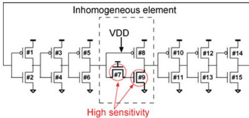
Fig. 6. Proposed pass-gate-based inverter structure for inhomogeneous element. RO frequency is sensitive to the nMOSFETs of the inhomogeneous stage only.
