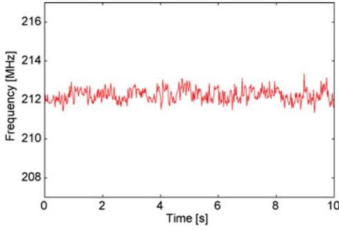
Fig. 13. RO frequency for an “INV-NPASS-I” inhomogeneous RO circuit over 10 s with small fluctuation (random noise) at 0.8 V supply.
