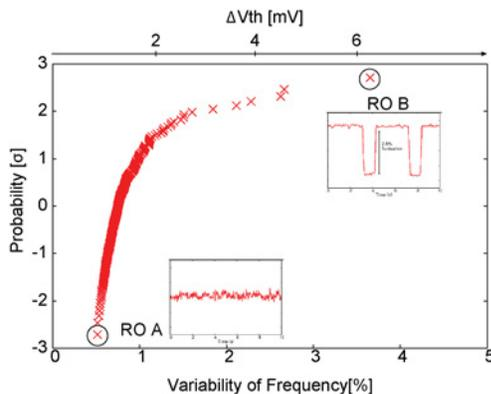
Fig. 24. CDF of RTN-induced threshold voltage variability.
