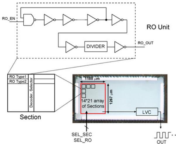
Fig. 9. Test structure to evaluate WID and RTN variability. Identical ROs are placed in an array of  $14 \times 21$ .
