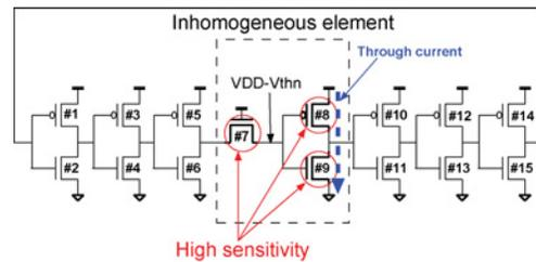
Fig. 4. Conventional pass-gate loaded inverter structure to create inhomogeneous element. RO frequency is sensitive to the three transistors in the inhomogeneous stage.
