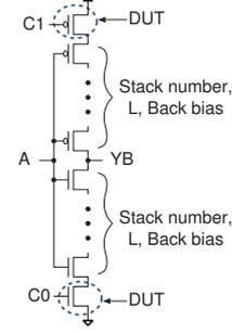
Fig. 2: Reconfigurable leakage monitor cell.
