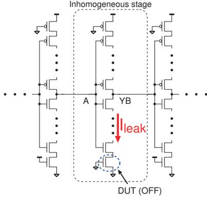
Fig. 4: Inhomogeneous structure to monitor single nMOSFET leakage current.
