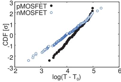
Fig. 8: CDF of WID leakage variation for nMOSFET and pMOSFET. The distribution fits log-normal distribution.
