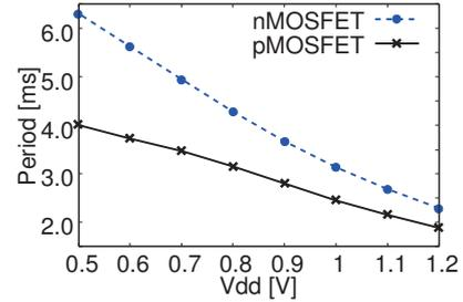
Fig. 10: Measured oscillation period due to  $N$  MOSFETs' leakage current at different supply voltages.
