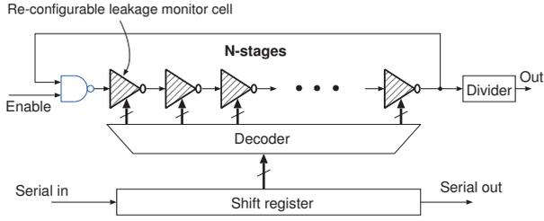
Fig. 3: Schematic of the reconfigurable leakage variation sensor circuit.
