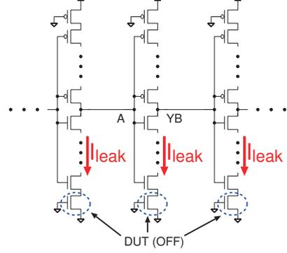
Fig. 5: Homogeneous structure to monitor average nMOSFET leakage current.
