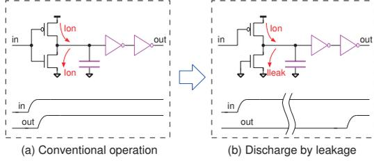
Fig. 1: Concept of converting leakage current to delay.
