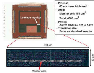
Fig. 6: Test chip micrograph and layout of the leakage variation sensor.
