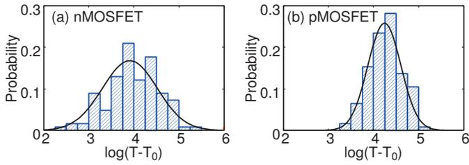
Fig. 7: Distribution of WID leakage variation. (a) nMOSFET, (b) pMOSFET. Log-normal distribution is observed.
