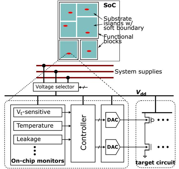
Fig. 2. A generic system architecture for energy optimization and variability resiliency with substrate islands.
