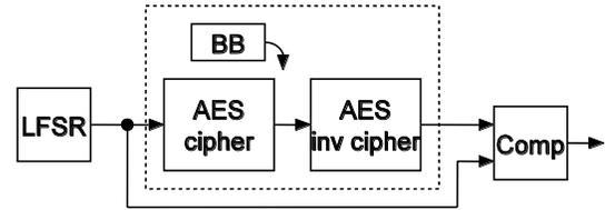
Fig. 10. Block diagram of self-testing module consisting of AES cipher and decipher modules.
