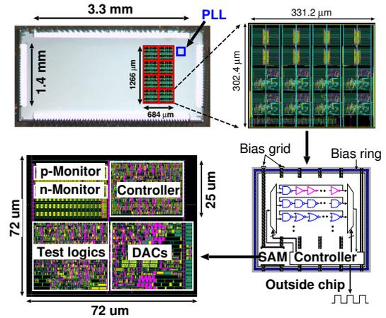
Fig. 7. Layout of the implemented on-chip monitoring and compensation scheme in a 65 nm process.
