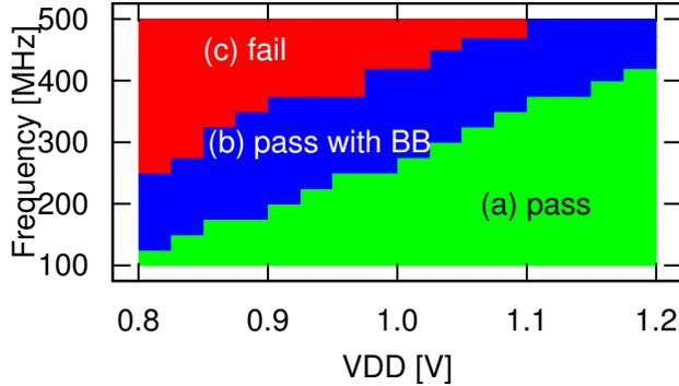
Fig. 12. Shmoo plot of the AES cipher/decipher self-testing module. Maximum of 0.6 V of forward body bias is applied.
