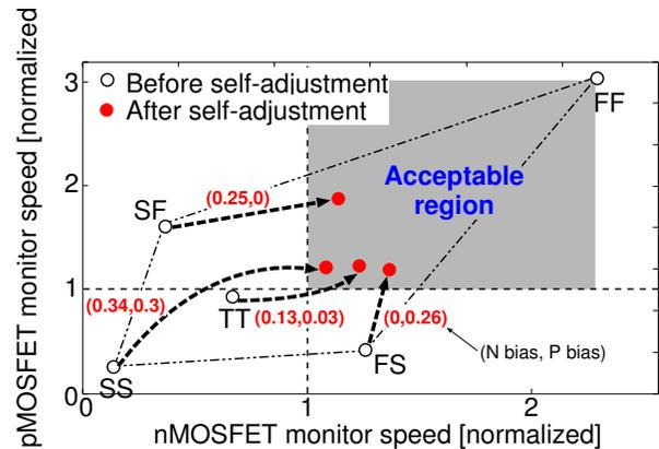
Fig. 8. Output performances of pMOSFET-sensitive and nMOSFET-sensitive ROs. Performances are measured before and after self-adjustment. Generated body biases for each corner are shown in the closed brackets.
