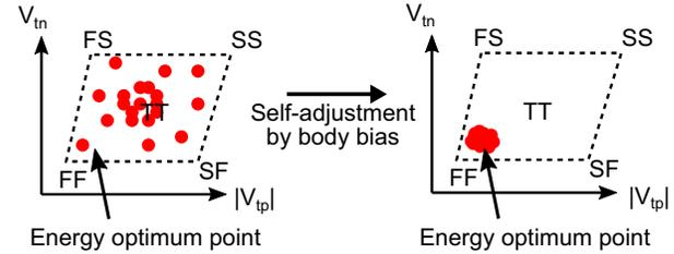
Fig. 4. Concept of self-adjustment of device threshold voltages to their energy-optimum values.
