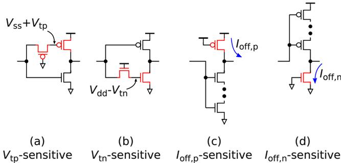
Fig. 3.  $V_t$ - and leakage-sensitive inverter delay cells.
