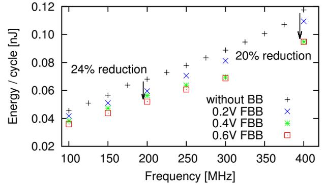
Fig. 13. Energy per cycle versus operating frequency with and without body bias tuning.
