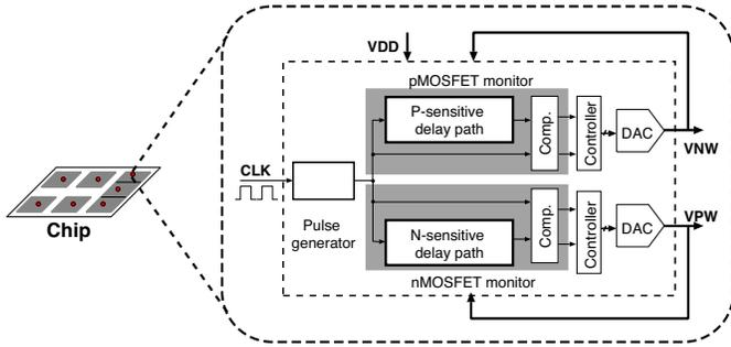
Fig. 5. On-chip fine-grain process variation compensation using separate pMOS- and nMOS-sensitive delay paths.
