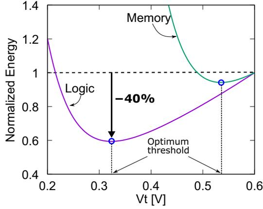
Fig. 1. Energy consumption of logic circuit and memory circuit against threshold voltage under a fixed delay constraint.
