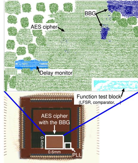
Fig. 11. Layout of an AES cipher and decipher module with built-in monitors and body bias generators.
