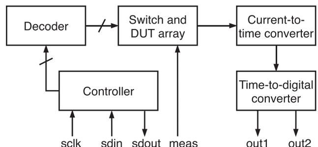
Fig. 5. Block diagram of proposed current measurement flow.
