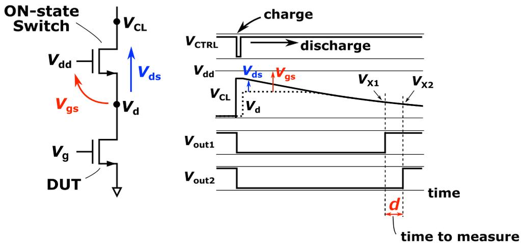
Fig. 2. (Color online) The ON-state switch transistor in the MOSFET selection circuit (left) and voltage waveform of current-to-time converter (right).
