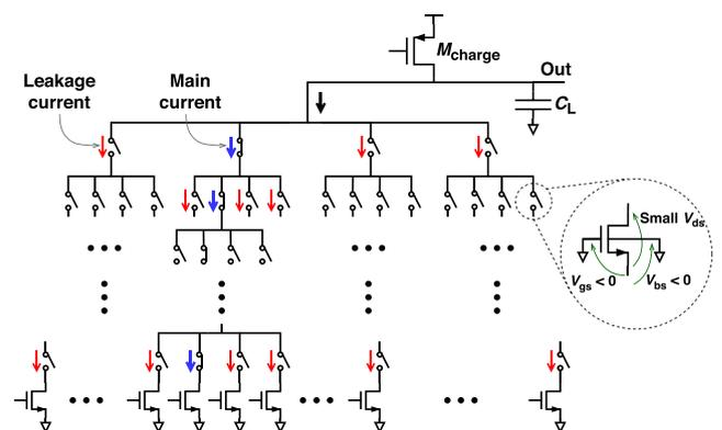
Fig. 4. (Color online) Tree structure of switches to reduce unwanted leakage current.
