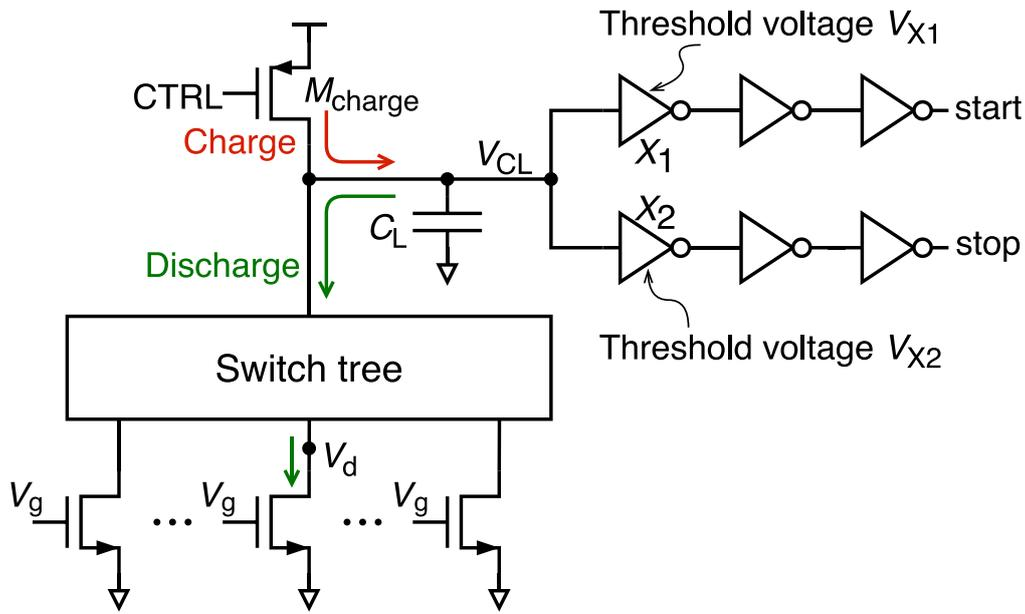
Fig. 1. (Color online) Topology of our proposed compact current-to-time converter.
