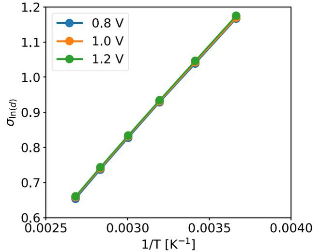
Fig. 8. (Color online) Standard deviation of the logarithm of measured delay against temperature for three different supply voltages of 0.8 V, 1.0 V and 1.2 V when V<sub>g</sub> = 0.2 V.
