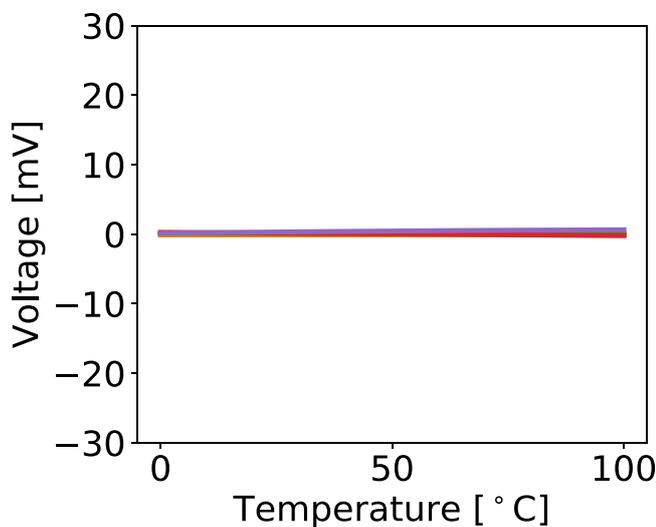
Fig. 3. (Color online) Deviation of logic threshold different at different temperatures and different process corners.
