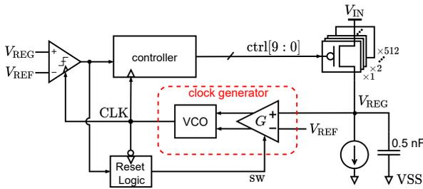
**Fig. 2:** Block diagram of the proposed LDO.
