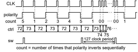
Fig. 5: Timing chart of control and reset logic.
