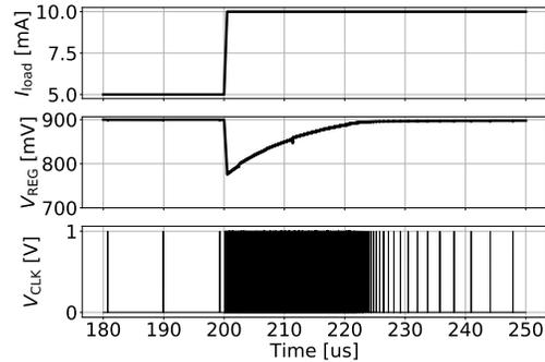
Fig. 9: Transient response with a 5–10 mA load change in 500 ns.
