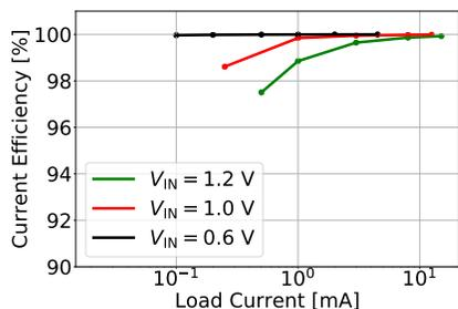
Fig. 10: Current efficiency at 0.1 V dropout.
