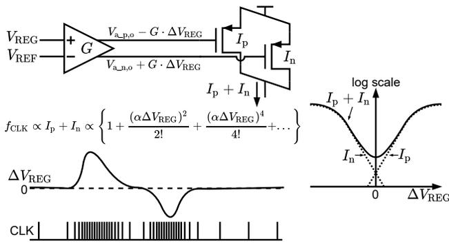
**Fig. 1:** Operating principle of non-linear frequency modulation ( $\alpha = G/(nV_T)$ ).
