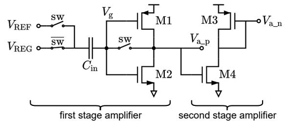
**Fig. 3:** Schematic of preamplifier.
