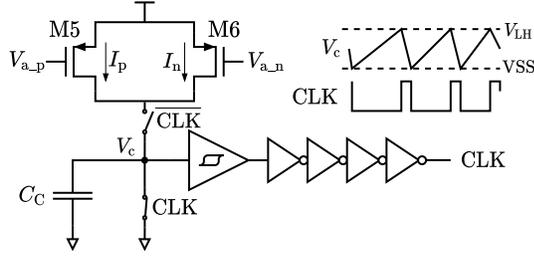
Fig. 4: Relaxation oscillator based non-linear VCO.
